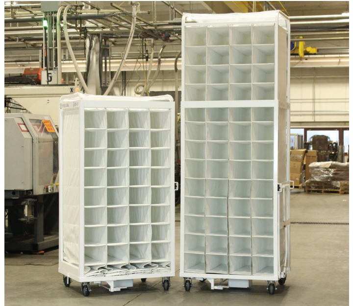
RZR Rack in lowered position (left) and RZR Rack raised to full storage capacity (right).
